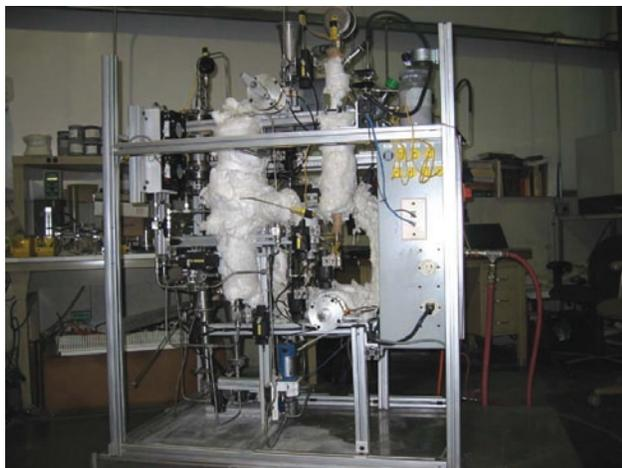
FIGURE 2. Mixer Showing Reactor and Pumps
