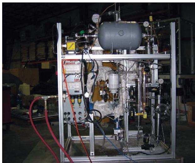
FIGURE 3. Mixer Showing H<sub>2</sub> and Water Control Systems
