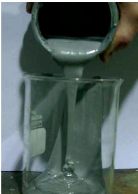
FIGURE 1. 70% Magnesium Hydride Slurry
