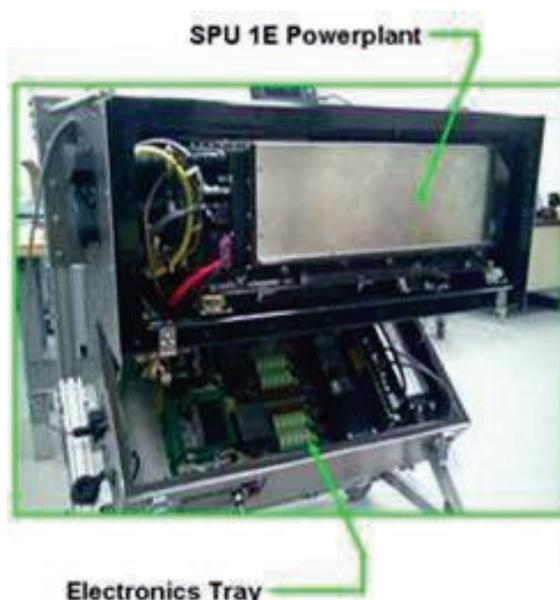
FIGURE 2. Electronics Tray Integrated with the SPU-1E Powerplant
