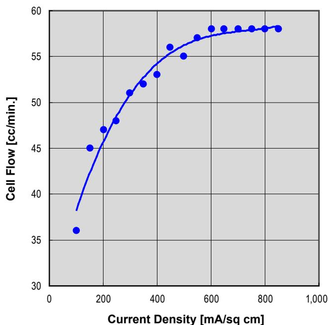
**FIGURE 2.** Cathode-Feed (Non-Pumped) 160 cm<sup>2</sup> Single-Cell Water Circulation Rate
