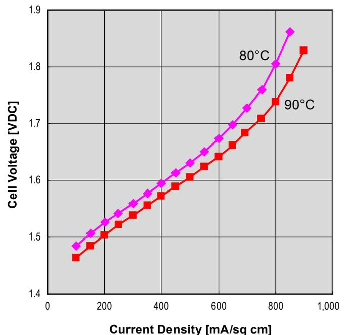
**FIGURE 3.** Cathode-Feed (Non-Pumped) 160 cm<sup>2</sup> Single-Cell Polarization Testing
