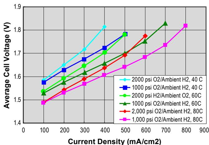
FIGURE 4. Cathode Feed (Pumped) Nafion® 117 Operation
