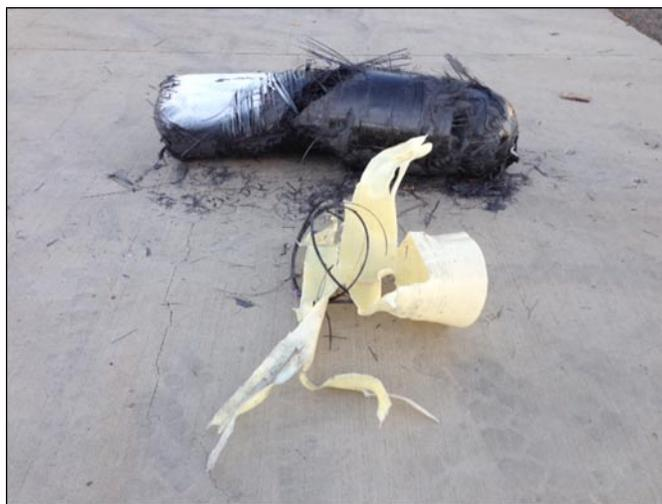
FIGURE 2. Vessel 15 Post Burst Test
