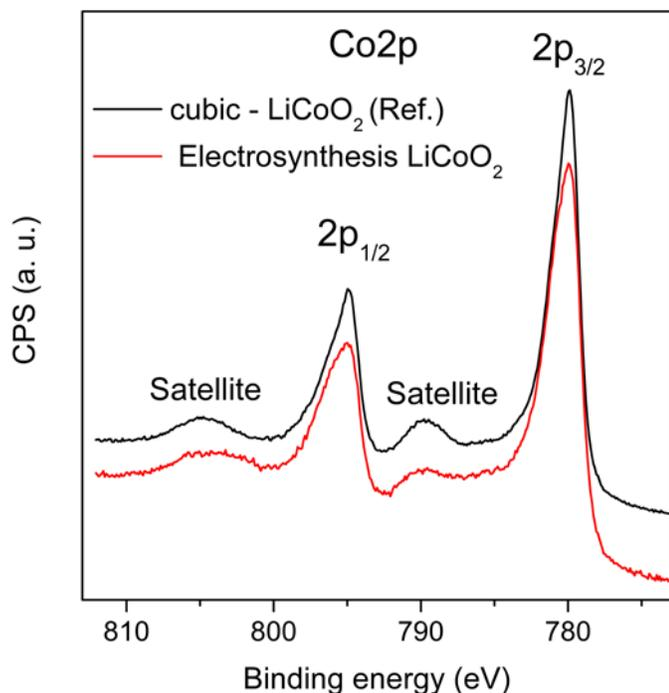
**FIGURE 4.** X-ray photoemission  $\text{Co}_{2p}$  spectra of cubic -  $\text{LiCoO}_2$  and electrosynthesis  $\text{LiCoO}_2$ .  $2p_{3/2}$  (780 eV) and satellite peaks (790 eV) are attributed to  $\text{Co}^{3+}$ .
