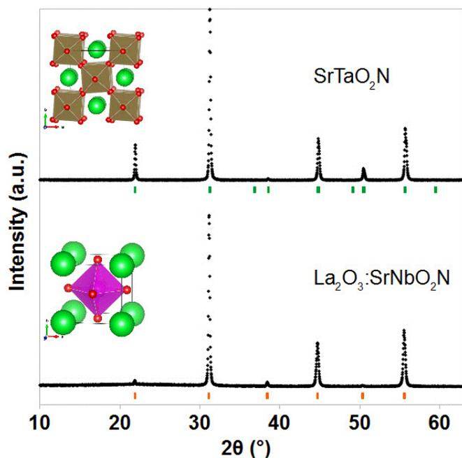
**FIGURE 2.** Laboratory X-ray powder diffraction for SrTaO<sub>2</sub>N (black dots; top) and La<sub>2</sub>O<sub>3</sub> doped SrNbO<sub>2</sub>N (black dots; bottom) are matched to indexed peaks (green and orange ticks). Each structure (insets) contains Sr (green spheres), O/N (red), and a B-site cation (Nb = purple polyhedron, Ta = tan polyhedron).
