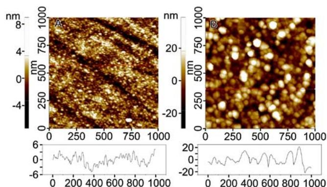
**FIGURE 3.** AFM image of (a) bare glassy carbon (GC) and (b) Sr<sub>2</sub>Nb<sub>2</sub>O<sub>7</sub> thin film deposited by PLD and line profile. Roughness of (a) and (b) are 1.3 nm and 7.8 nm, respectively.
