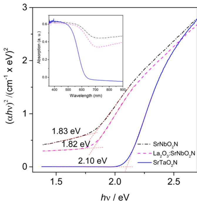
**FIGURE 1.** Tauc plot of SrNbO<sub>2</sub>N, 5 mol% doped SrNbO<sub>2</sub>N, and SrTaO<sub>2</sub>N. Bandgap values of SrNbO<sub>2</sub>N, 5 mol% doped SrNbO<sub>2</sub>N, and SrTaO<sub>2</sub>N were obtained as 1.83 eV, 1.82 eV, and 2.10 eV, respectively (UV-VIS diffuse reflectance spectra).
