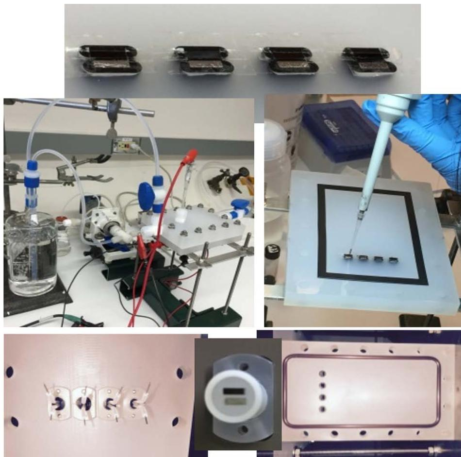
**FIGURE 1.** Pictures of the Eiya m-CFDE, cell showing the glassy carbon and platinum electrodes imbedded in the cell wall, and of the ANL m-CFDE showing the electrodes imbedded in removal “plugs”
