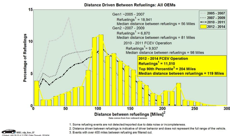
**FIGURE 4.** FCEV actual driving distance between refueling trend and comparison
