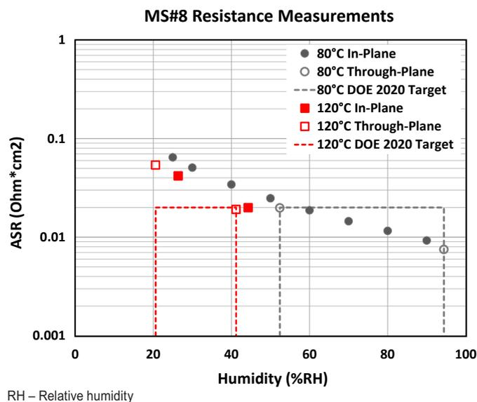
**FIGURE 2.** Area specific resistance vs. relative humidity measured through-plane (open symbols) or calculated from in-plane conductivity (filled symbols) for Milestone 8 membrane measured at 80°C and 120°C. DOE targets are shown in dashed lines.
