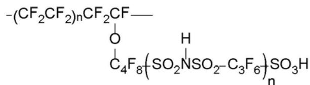
**FIGURE 1.** Ionomer with bis(sulfonyl)imide and sulfonic acid side chain. The ionomer is designated PFIA when n = 1 and PFICE when n > 1.
