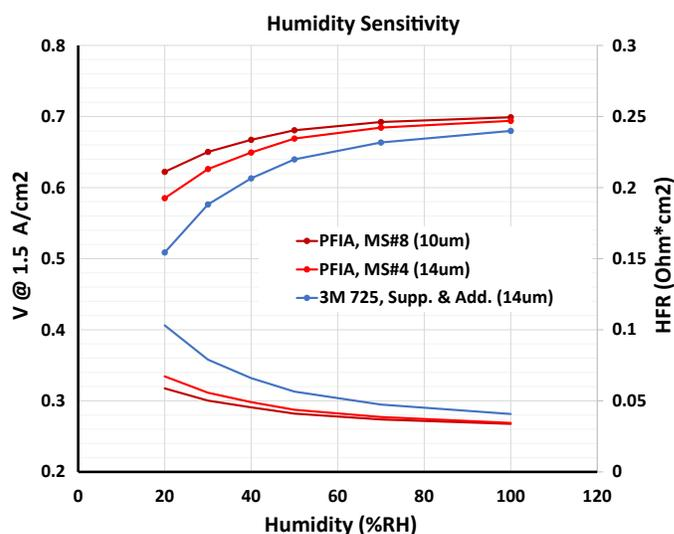
**FIGURE 3.** Voltage and high frequency resistance (HFR) for Milestone 4 and 8 membranes, as a function of humidity at 1.5 A/cm<sup>2</sup>.
