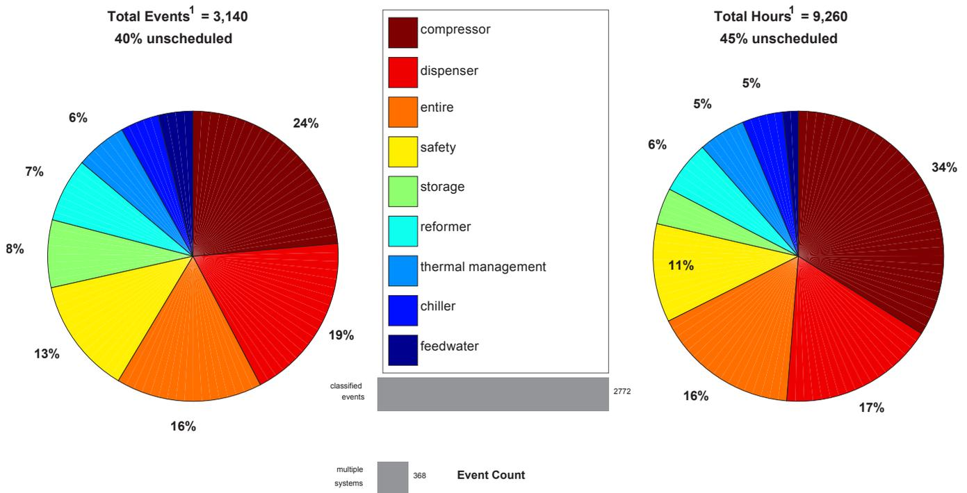
FIGURE 4. Maintenance by equipment type
