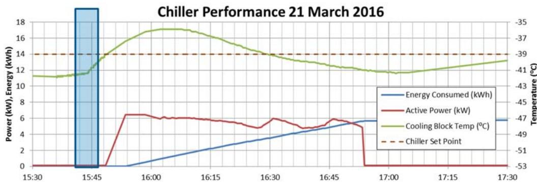
**FIGURE 3.** Chiller performance data showing the power (red line) and energy (blue line) requirements to recover the heat exchanger block temperature (green line) from a fill (indicated by the blue shaded rectangle). The system is unable to perform a fill when the cooling block temperature is above the set point (orange dotted line).
