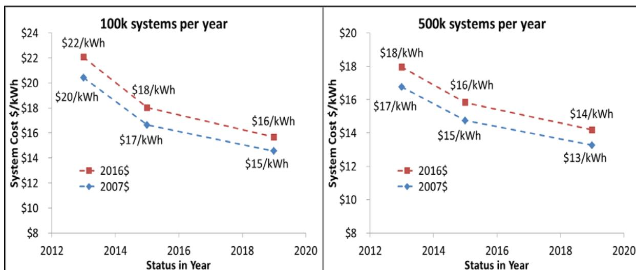
Figure 3. Comparison of storage system cost status in 2007 U.S. dollars (2007\$) and 2016 U.S. dollars (2016\$) as reported in 2013,<sup>3</sup> 2015,<sup>4</sup> and 2019. Costs are for annual productions of 100,000 units (left) and 500,000 units (right).
