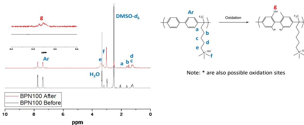
Figure 2. <sup>1</sup>H NMR change of the BPN ionomer before and after 100-hour MEA test at 2.1 V vs. RHE
