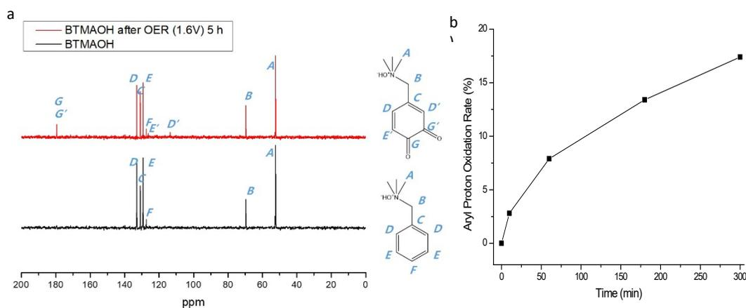
**Figure 1. (a) <sup>1</sup>H NMR change of the BTMAOH electrolyte before and after 5-hour IrO<sub>2</sub> RDE test at 1.6 V vs. RHE (b) Aryl proton oxidation rate of BTMAOH as a function of time**
