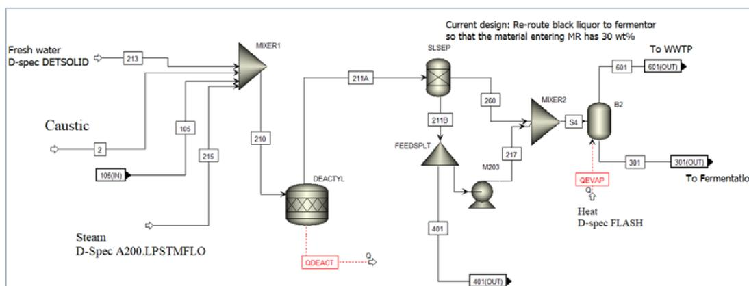
Figure 5. The flow scheme for corn stover pretreatment
