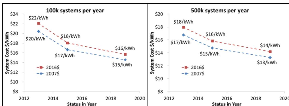
Figure 4. Comparison of storage system cost status in 2007\$ and 2016\$ as reported in 2013 [13], 2015 [14], and in 2019. Costs are for annual productions of 100,000 units (left) and 500,000 units (right).
