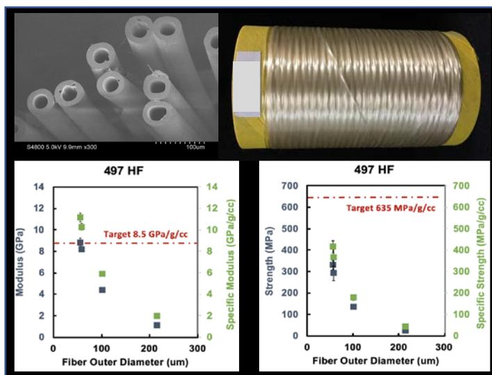
Figure 1. Scanning electron microscopy image of TechPAN precursor hollow filament cross sections and tensile results for hollow precursor fibers spun with varying ODs. ( $N = 25$  for each point, 25.4 mm gauge length, all tensile measurements based on force per area defined by the hollow fiber OD, density based on mass per volume defined by the hollow fiber OD)
