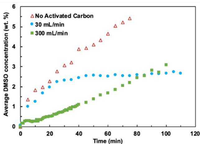
**Figure 3. Comparison of the average DMSO concentration in the bath vs. spinning time for three solvent recovery conditions: no activated carbon, 30 mL/min through AC, and 300 mL/min through AC. Standard air gap spinning of 100-filament TechPAN tow. (2.8 L water-solvent total, 480 g of AC—up to 0.18 g DMSO per 1 g AC, 0.05 kg precursor spun)**
