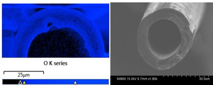
**Figure 2. (Left) EDS image of an oxidized hollow PAN fiber showing oxygen content (blue), demonstrating oxidation is occurring from both the interior lumen of the fiber as well as the exterior. (Right) Cross section of a hollow carbon fiber produced at University of Kentucky Center for Applied Energy Research.**
