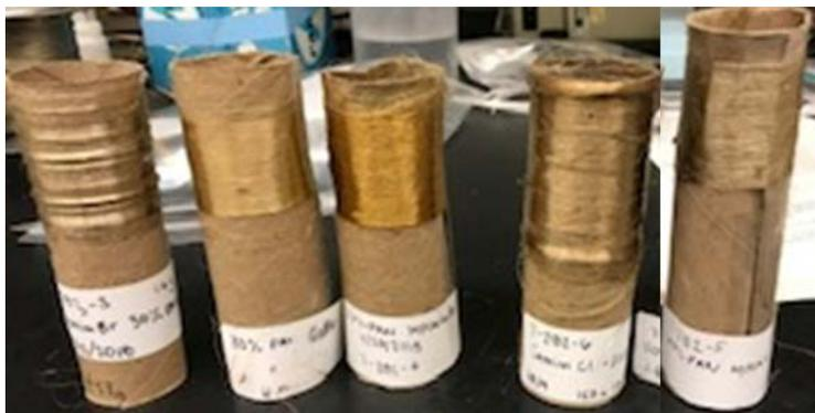
Figure 2. Melt spun PAN fiber from PAN-IL composites containing [C<sub>3</sub>mim]Br, [C<sub>4</sub>mim]Br, [MPCNIm]Br, [C<sub>4</sub>mim]Cl, and [MPCNIm]Cl in order from left to right
