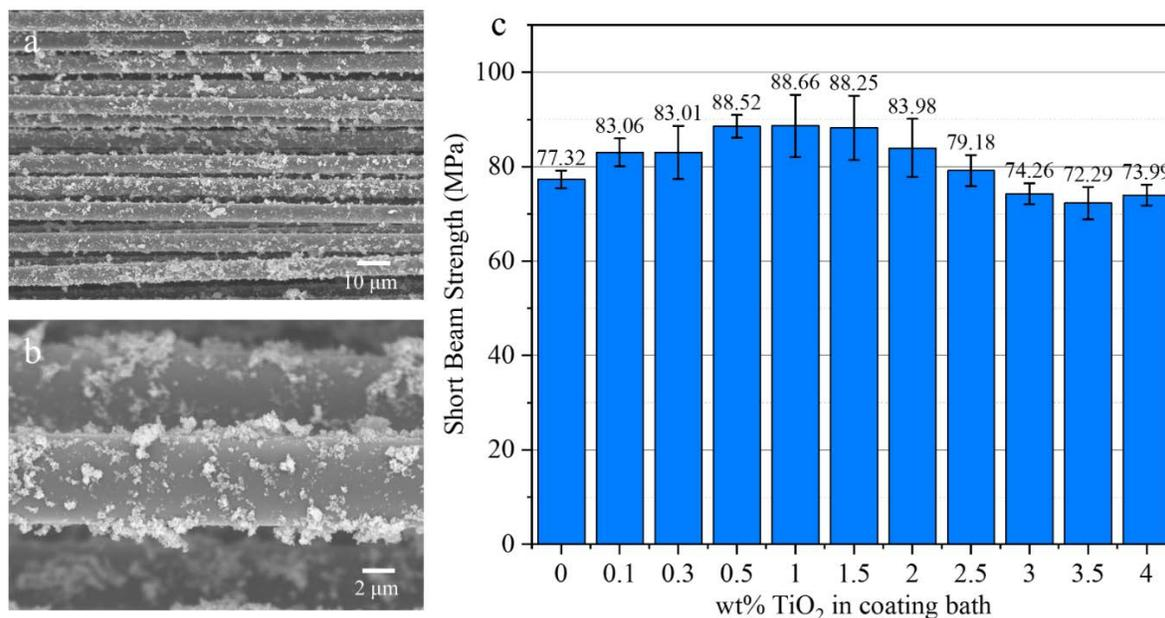
Figure 2. (a-b) Scanning electron microscope images of TiO<sub>2</sub> nanoparticle coated carbon fibers with (c) the corresponding results of the short beam shear tests as a function of the concentration of nanoparticles in the coating bath.
