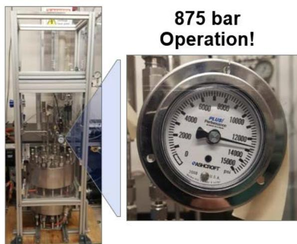
**Figure 3. EHC stack operating at 875 bar**
