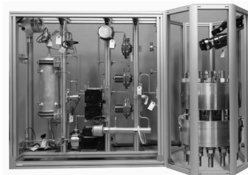
Figure 4. 875-bar EHC system assembly
