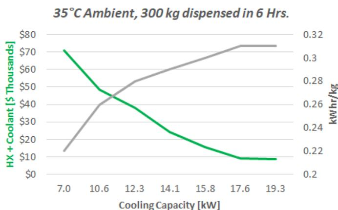
Figure 3. Modeling of capital cost (heat exchanger plus brine coolant) and operating cost (kWh per kg hydrogen dispensed) versus chiller capacity, based on a single-nozzle installation
