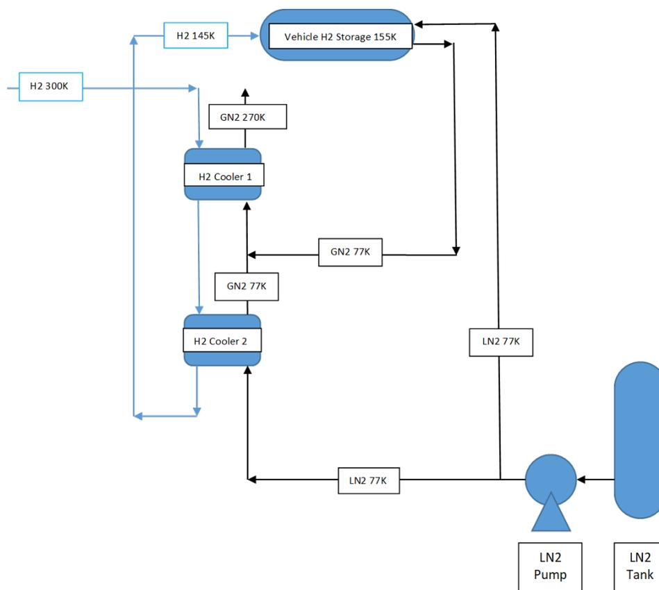
Figure 2. Cooling equipment configuration at a hydrogen refueling station that requires LN<sub>2</sub> temperature cooling of both hydrogen gas and onboard storage tank
