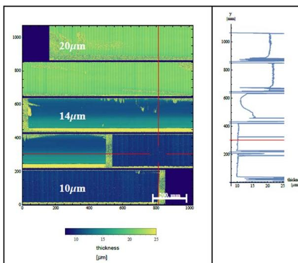
Figure 1. Membrane thickness imaging data from web-line run
