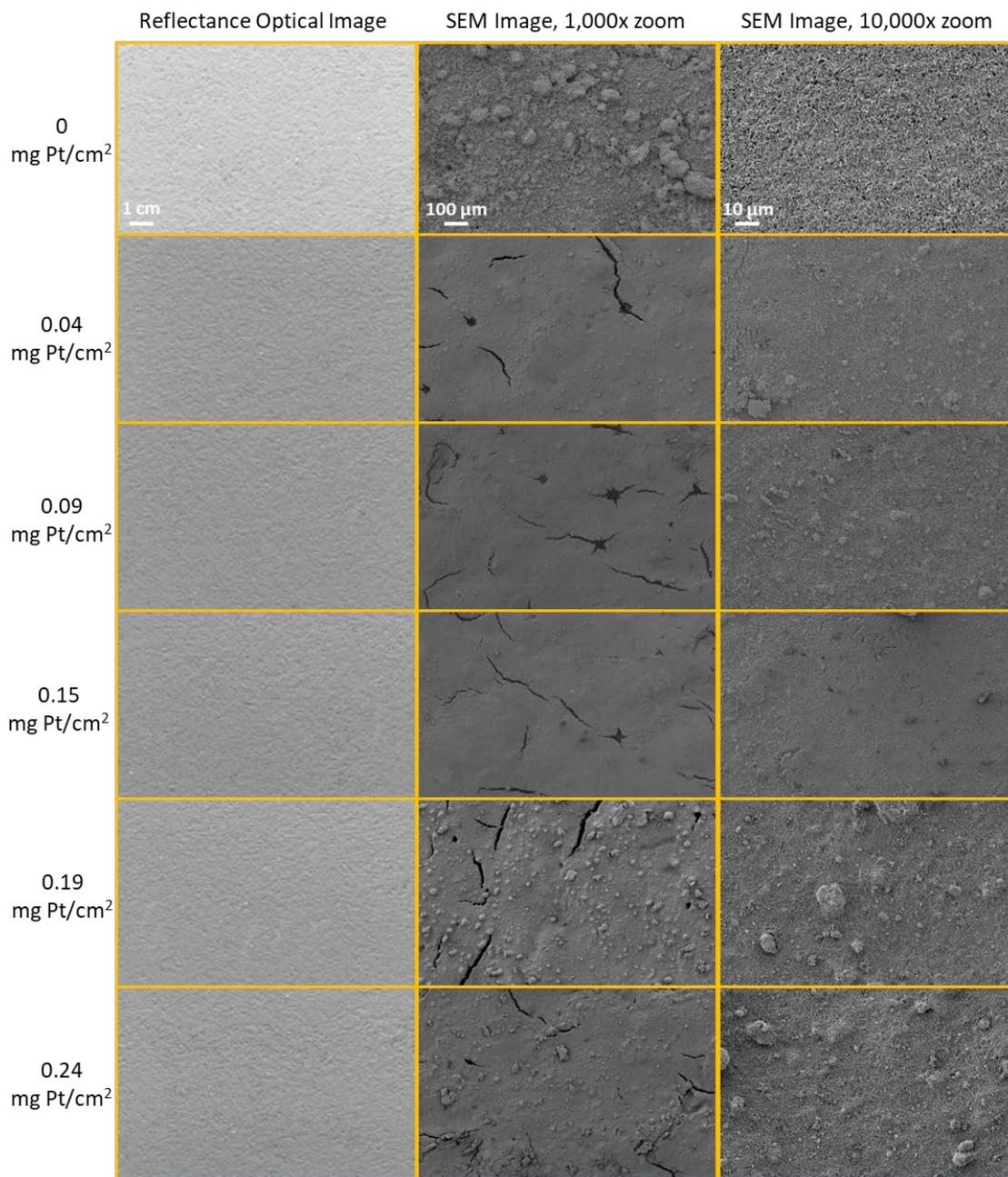
Figure 3. Comparisons of GDLs loaded with 0–0.24 mg Pt/cm<sup>2</sup> taken by optical reflectance and different magnifications of SEM to show the difference in observable surface features
