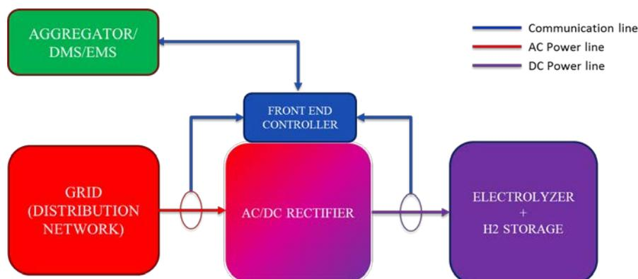
**Figure 1. Experimental setup for FEC with hydrogen electrolyzer**
