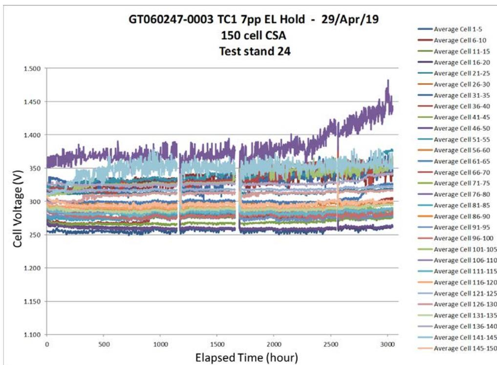
Figure 3. The 150-cell CSA stack produced 5.5 kg/day hydrogen at 0.5 A/cm<sup>2</sup> and verified performance degradation of less than 1%/1,000 h for a period of nearly 3,000 h
