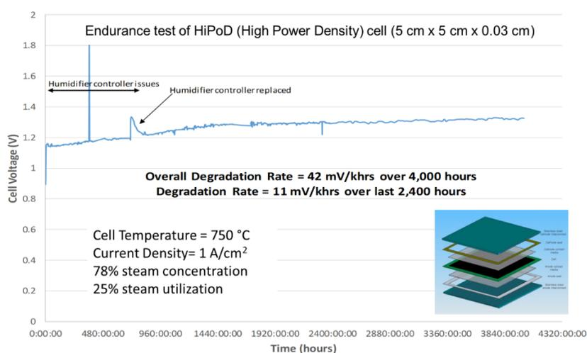
**Figure 1. Test of HiPoD cell (5 cm x 5 cm x 0.03 cm) at  $1 \text{ A/cm}^2$  demonstrated voltage degradation rate of less than  $1\%/1,000 \text{ h}$  over the last  $\sim 2,400 \text{ h}$  of operation**
