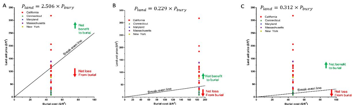
Figure 4. Comparison of burial cost and land unit price for (A) gaseous hydrogen underground direct-bury, with burial cost estimated at \$45.8/ft²; (B) gaseous hydrogen underground vault design, with underground vault cost estimated at \$185.0/ft²; and (C) liquid hydrogen underground direct-bury design, with burial cost estimated at \$45.8/ft²
