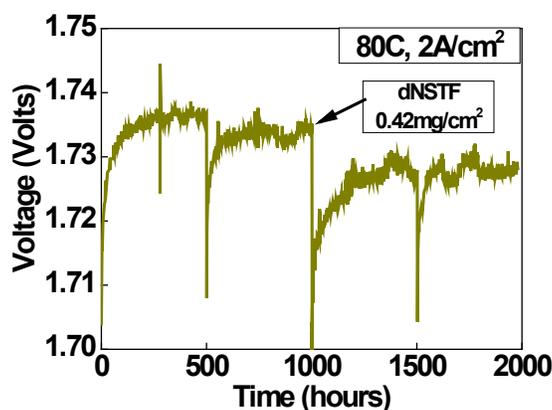
Figure 9. PEMWE durability test of dispersed Ir/NSTF anode with 0.42 mg-Ir/cm<sup>2</sup> loading
