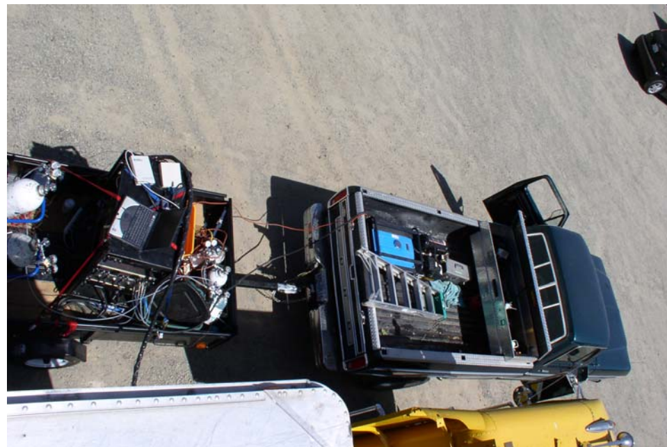
Emissions sampler as seen from the top of the large trailer unit.
