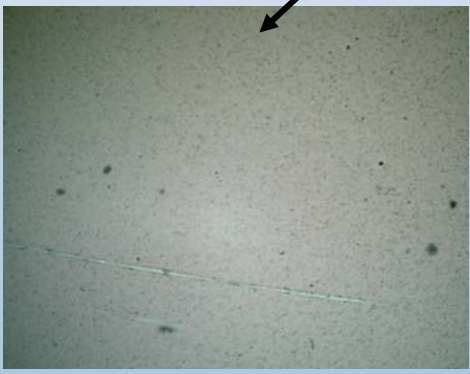
Fair quality electrodeposited CGS film on Mo substrate
