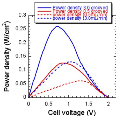
**FIGURE 3.** Power curves for flat and textured/grooved Pt electrodes for a planar membraneless fuel cell with  $0.15\text{M NaBH}_4$  in  $3\text{M NaOH}$  as fuel and  $0.5\text{M CAN}$  in  $1\text{M HNO}_3$  as oxidant.
