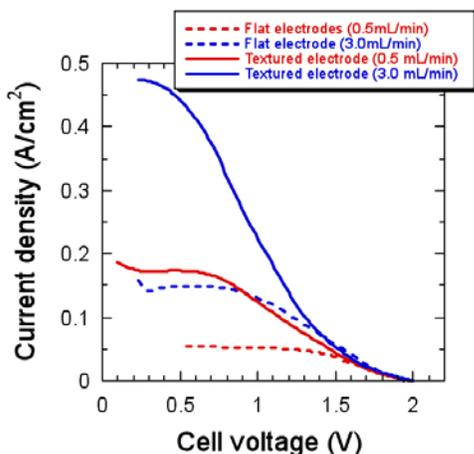
**FIGURE 2.** Load curves for flat and textured Pt electrodes for a planar membraneless fuel cell with  $0.15\text{M NaBH}_4$  in  $3\text{M NaOH}$  as fuel and  $0.5\text{M CAN}$  in  $1\text{M HNO}_3$  as oxidant and at flow rates of  $0.5$  and  $3.0 \text{ mL/min}$ .
