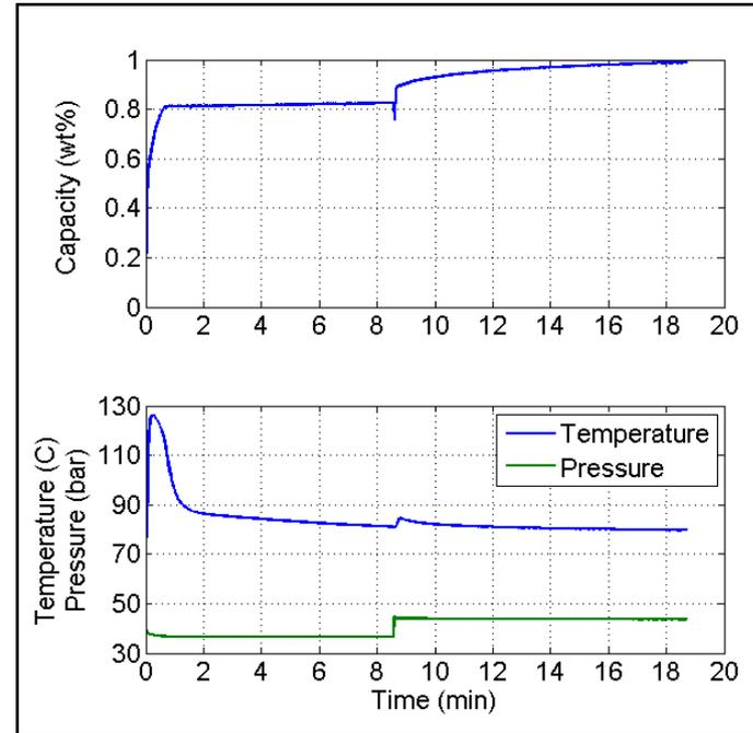
Absorption profiles for Hy-Stor 208.  $\text{MmAl}_{4.5}\text{Ni}_{0.5}$  at various pressures. Demonstration of rapid kinetics and acceptable H<sub>2</sub> capacity.
