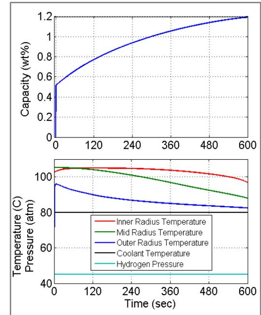
**Refueling Simulation Results Showing the Full 1.2 weight % of H<sub>2</sub> Absorbed in 10 min.**
