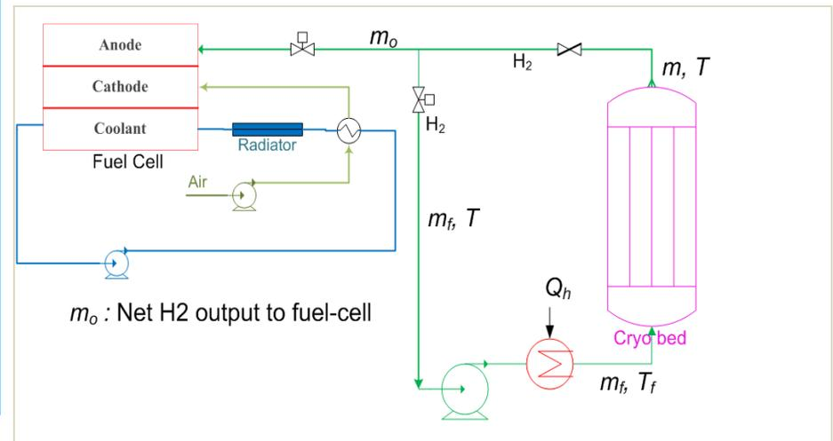
Cryo-adsorption Discharge Schematic Diagram with Hot Gas Recirculation
