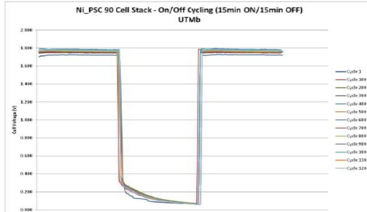
Electrolyzers demonstrate quick start-stop without degradation
