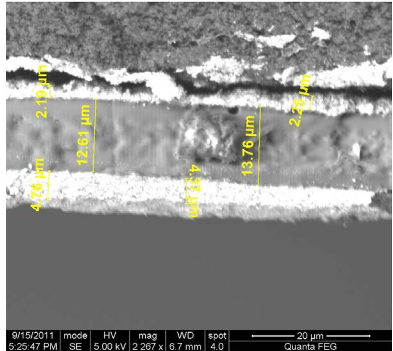
Pt band observed on cathode side of MEA. Band clearly visible after 2000 hours with high (0.4 mg.Pt/cm<sup>2</sup>) loaded catalyst
