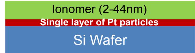
Model structure compatible with AFM, XPS, and SEM . . . not ideal for STEM-EELS.
