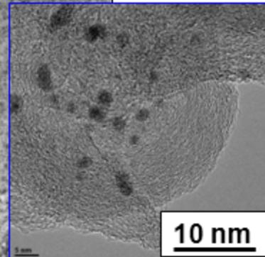
*After 100 hr at 1.2V, much of the HSAC has been oxidized to form graphite oxide*
