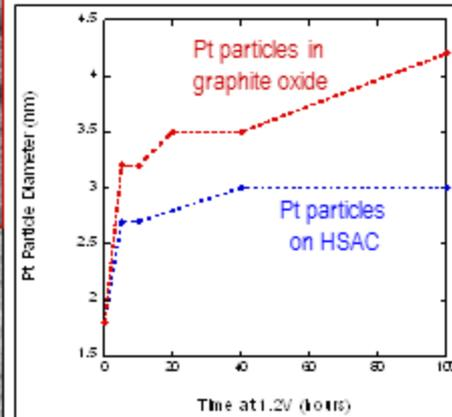
*After 100 hr at 1.2V, evidence for retained meso-graphitic HSAC structure*
