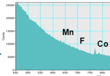
EELS spectrum from 2-3 nm thick ionomer layer. Fluorine peak is visible on first scan in thicker area, but disappears on second scan. No fluorine peak observed in first scan of thinner layer
