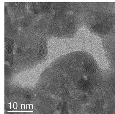
Samples not ideal for STEM-EELS analysis, since an etch in nitric acid required to remove Pt/Ionomer layer from Si.
