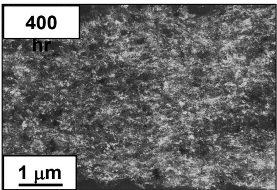
*Thinned cathode exhibits a "clustered" morphology of large Pt particles associated with localized graphite-oxide formation*
