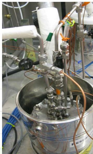
Integrated pressure vessel installed in experimental test loop
