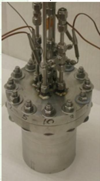
Fully assembled integrated pressure vessel
