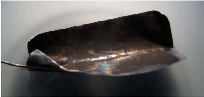
Platinum black counter electrode with shiny film due to durability testing
