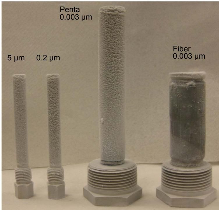
Warming up in air after immersion in liquid N<sub>2</sub>
