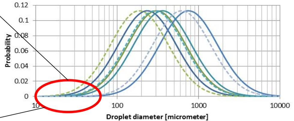
The small droplets cause carryover in gas/liquid separator
