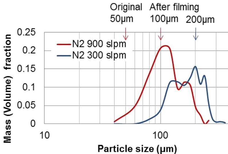
Filming inside the vortex finder is a mechanism that can generate droplets that are larger than the droplet size at the inlet of the vortex finder.
