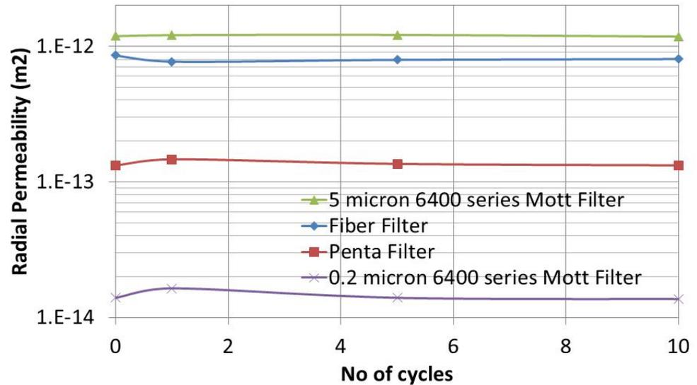
Resistant to thermal cycles between room temperature (RT) and 80K
