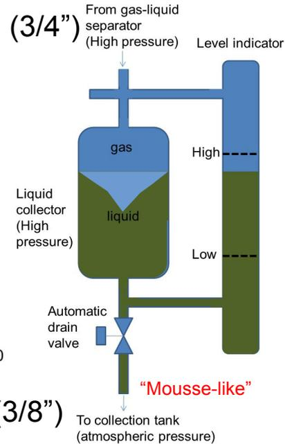
Drain system improved in order to maintain system pressure
