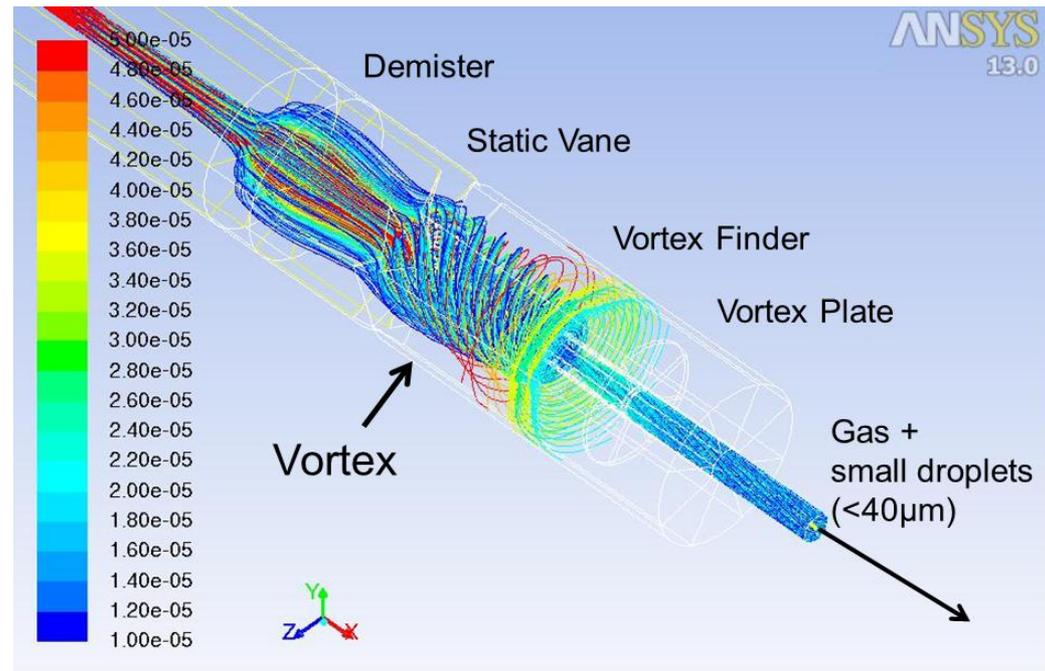
Small droplets (<50 µm) follow the streamlines of the gas
