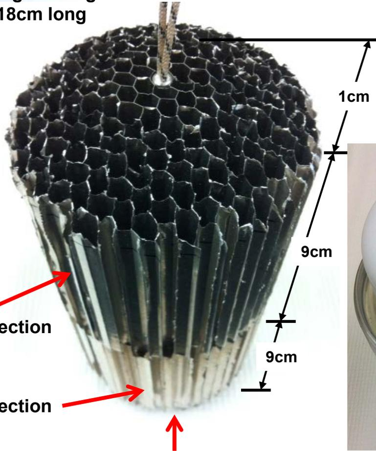
Heating cartridge is recessed by 0.8 inch (2cm) from the bottom hex-cell surface
