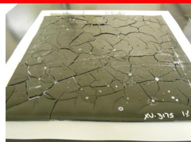
XV-3175 1%Asbury – cracking, white defects
