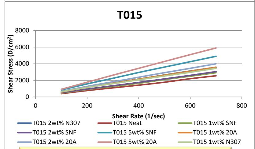
**T015 Resin system viscosity in range for filament winding**
