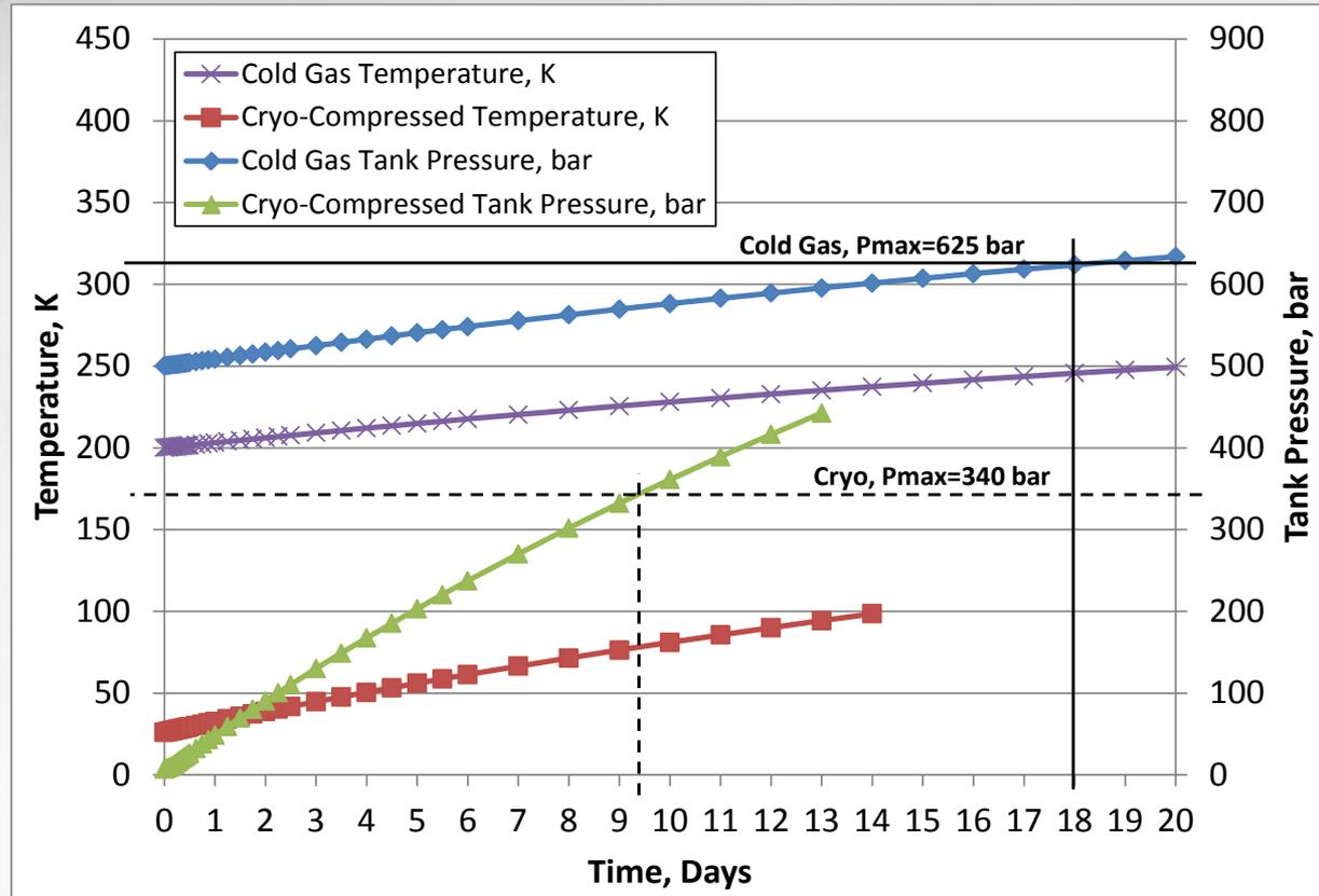
The cold gas storage with similar insulation to cryo-compressed can double the dormancy period
