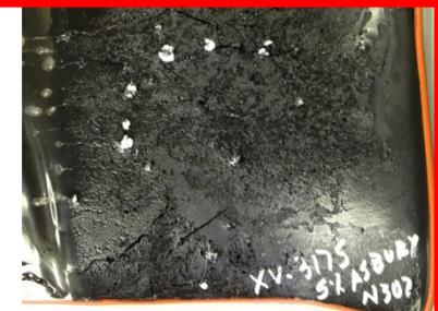
XV-3175 5%Asbury – cracking, white defects
