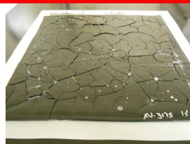
XV-3175 1%Asbury – cracking, white defects
