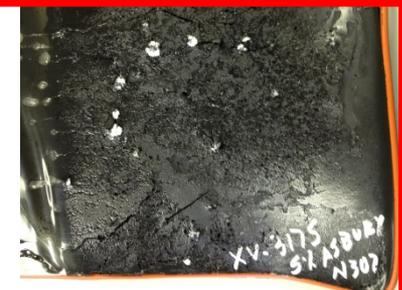
XV-3175 5%Asbury – cracking, white defects
