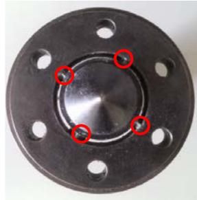
TLCP melt diverges radically from mandrel top, and splits at four spider support legs (circled with red).
