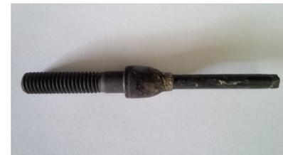
Air flows in from the air inlet on the mandrel, escaping from the air needle, inflating parison into the hollow mold.
