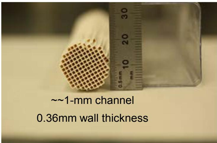
➤ Monolith integrity and porous structures are maintained at high calcination temperature
