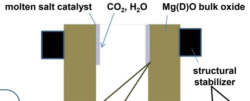
Catalyze gas/solid reaction during carbonation and decomposition
