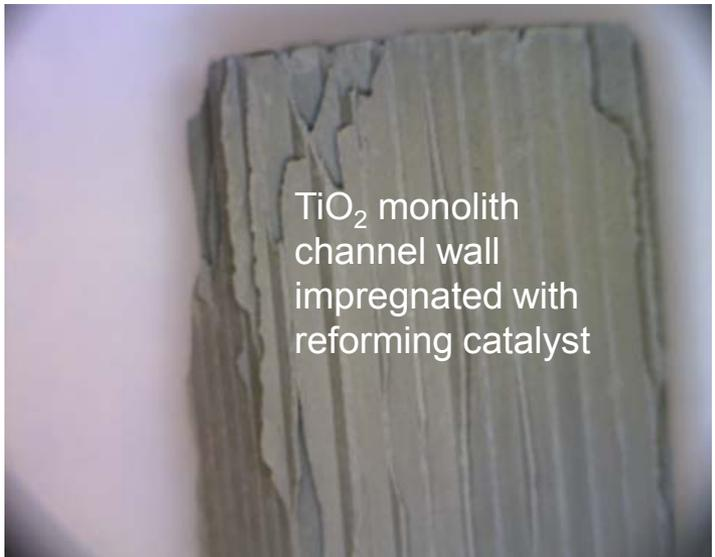
➤ Significant amounts of the catalyst can be loaded with uniform textures
