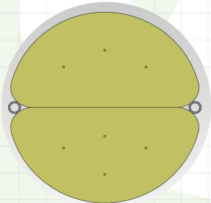
**Half-bed design is to maximize MOF-5 volume while enabling the assembly process**
