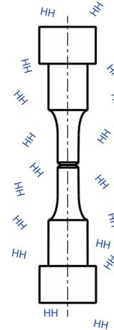
Notched tension-tension fatigue
