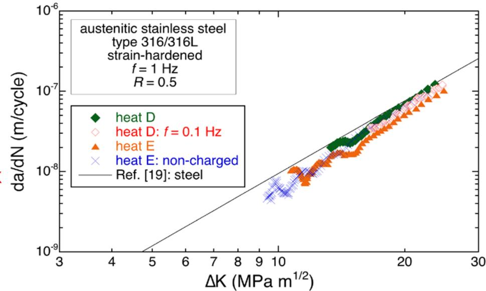
**Concern:** Fatigue crack growth design methodologies have not been implemented for design of manifold components.
