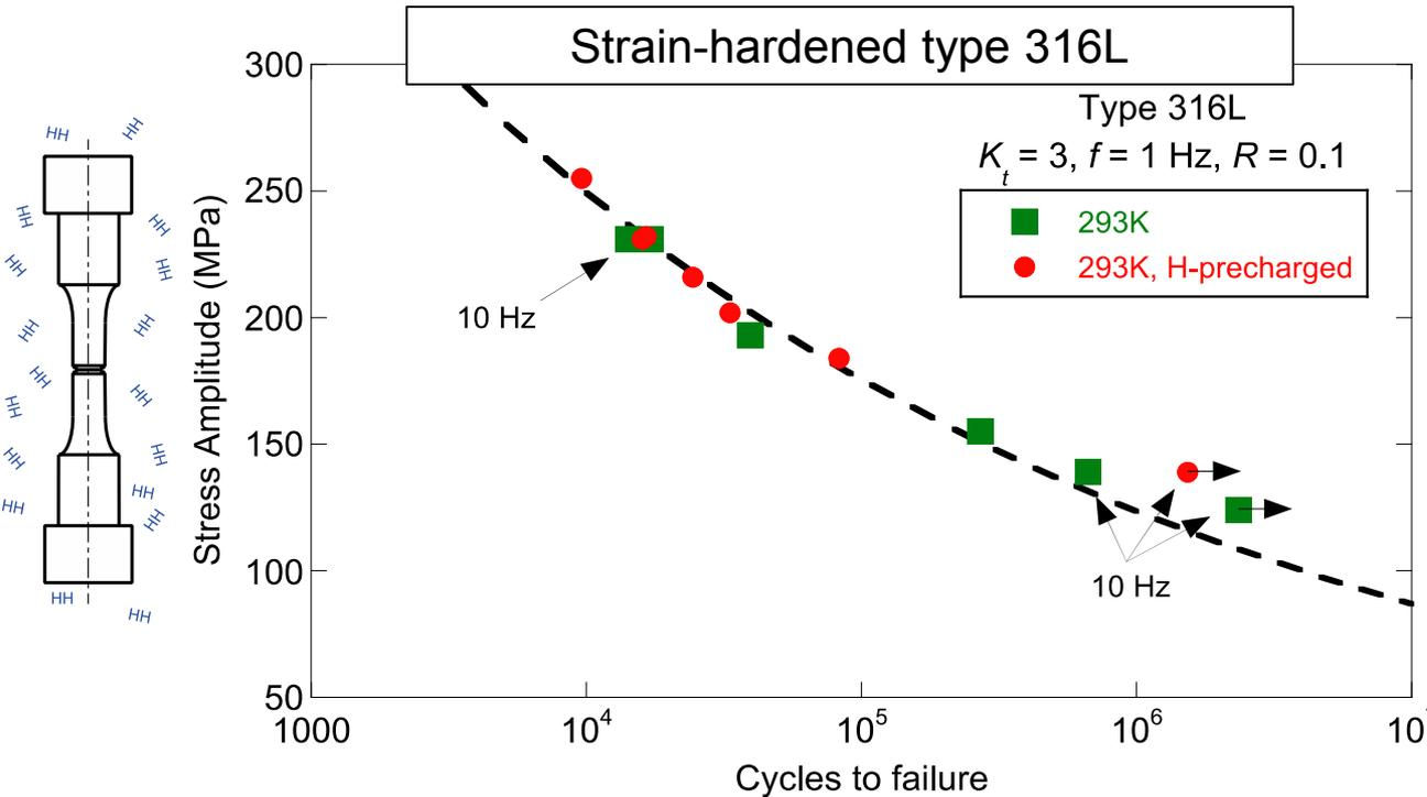
Notched tension-tension fatigue
