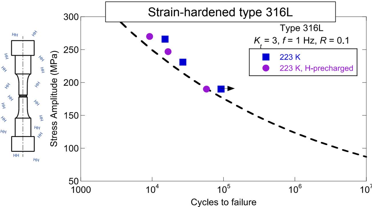
Notched tension-tension fatigue
