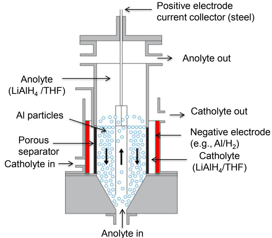
Simple design-cathodic LiAlH<sub>4</sub> degradation may cause issues
