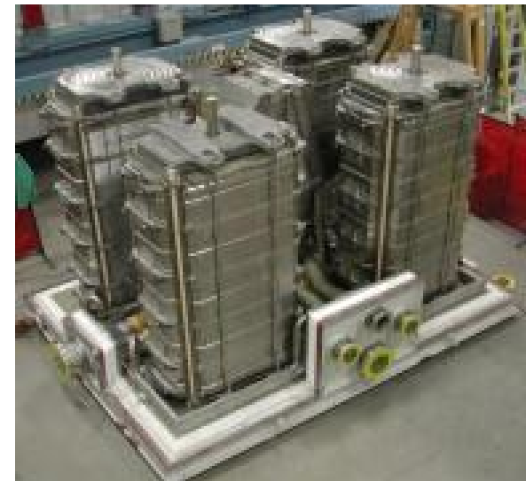
4 stacks are combined to build a 1.4 MW modules
