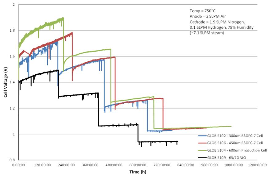
Comparison of Electrolysis Degradation Rate For 300, 450, 600 um Thick Cells and Modified Cathode Substrate Cell
