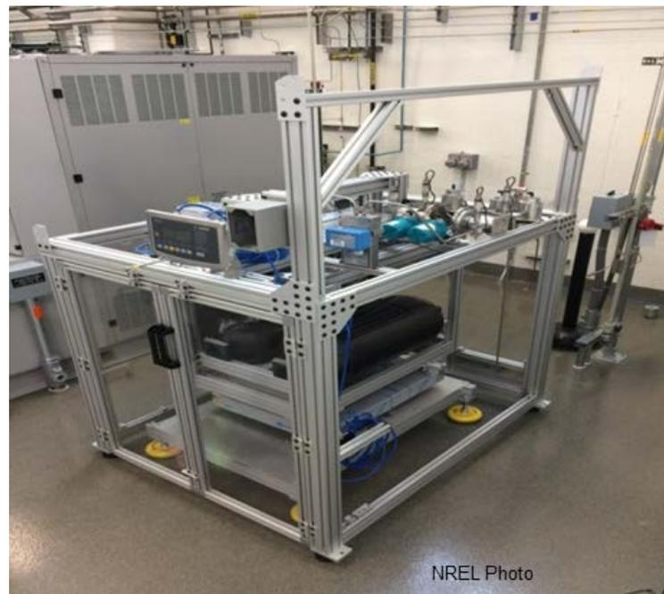
*NREL develops equipment to test accuracy of hydrogen flow meters for commercial sale of hydrogen (1.5% accuracy requirement).*
