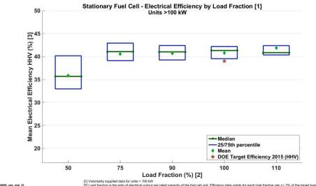
Electrical efficiency for fuel cells > 100 kW is 45% LHV and that exceeds the 2015 DOE technology validation target of 43% LHV (39% HHV) at load fractions over 50% (Results confirmed in April 2015 and December 2015 CDPs)
