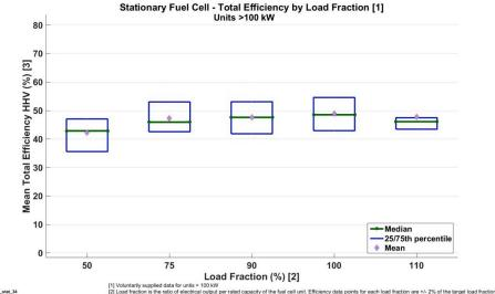
3] Mean total efficiencies by unit are calculated as the percentage of electrical plus heat outputs to higher heating value of fuel input. The natural gas higher heating value used is 48.956 MJ/kg and the lower heating value used is 44.294 MJ/kg.
