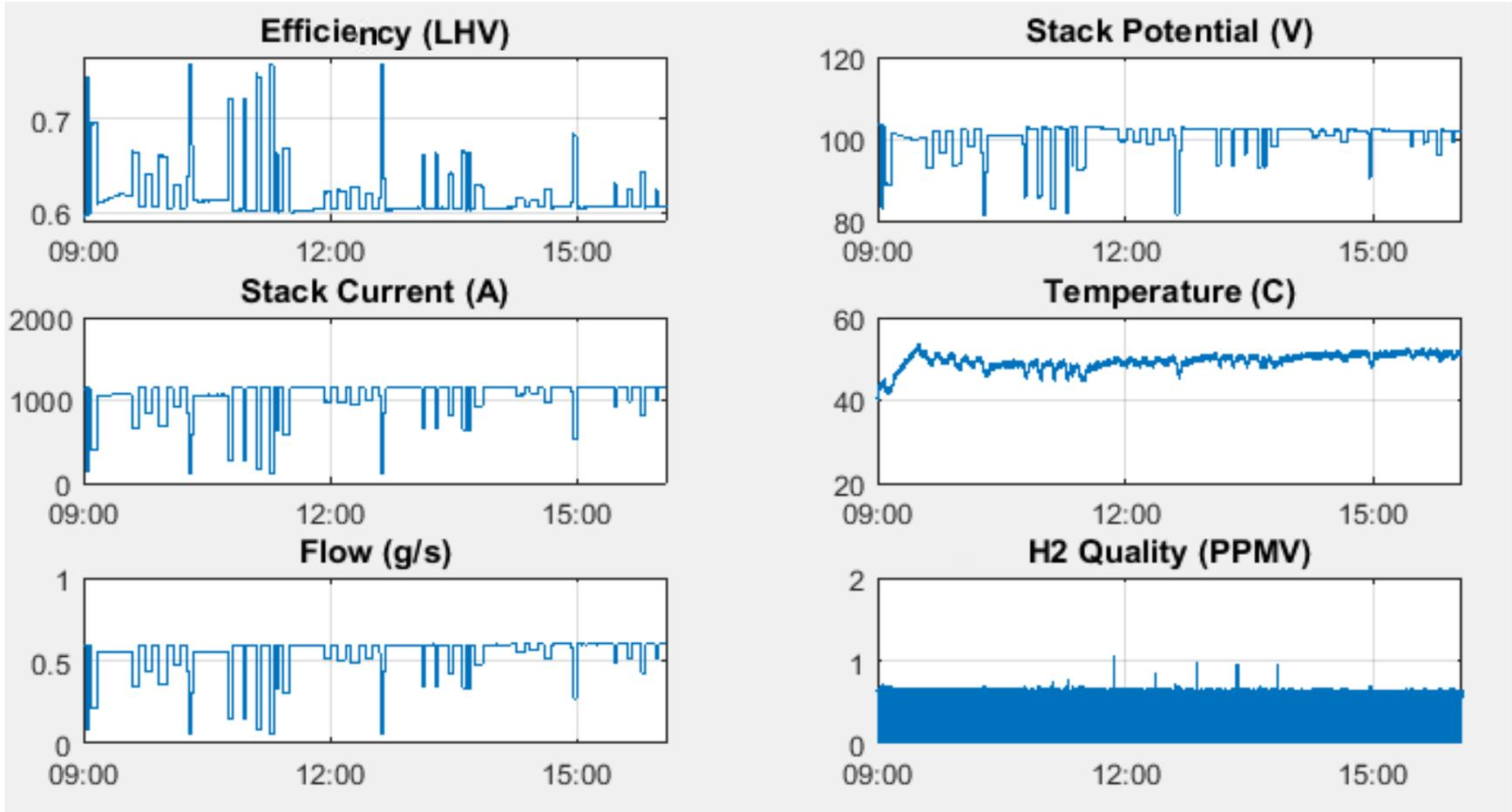
Stack performance data collected by the NREL SCADA system for PG&E E-20 profile
