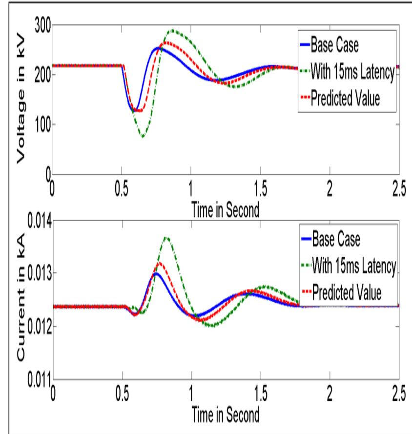
**Two phase to ground fault with Prediction**
