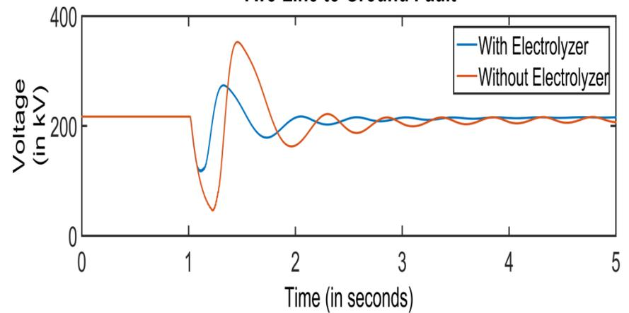
**Three Line to Ground Fault**
