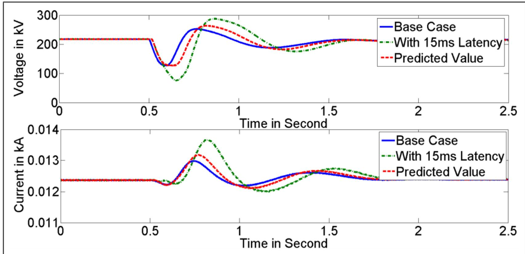
**Two phase to ground fault with Prediction**
