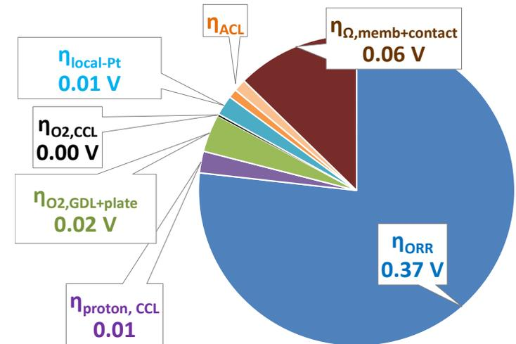
0.10 mg<sub>Pt</sub>/cm<sup>2</sup> PtCo/HSC: H<sub>2</sub>/air, 94°C, 250/250 kPa<sub>abs,out</sub>, 65/65% RH<sub>in</sub>, st=1.5/2
